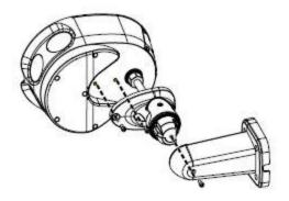
(2) Fix the bracket to the wall using four provided nails and flat washers.
