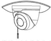
Adjust the monitoring direction, then tighten the screw.
